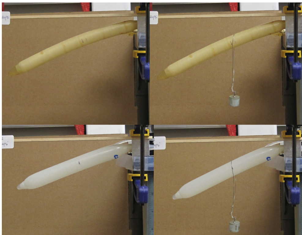
Figure 4. Unloaded and loaded cantilever testing of the 18-cm AMS 700 LGX and 18-cm Coloplast Titan. Figure 4 is available in color at www.jsm.jsexmed.org .
